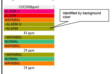
Fail: Gray Trouble Warning: Orange 1st alarm Alarm: Red: 2nd alarm AlarmH: Magenta 3rd alarm STEL: Pink STEL alarm TWA: TWA alarm Bright purple Alarms restored Olive Normal: Dark green All alarms restored Bright red Full-scale over Over:
