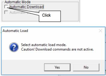
Click "Yes" to switch to automatic processing and to download data from the main unit automatically when communication is performed next.
