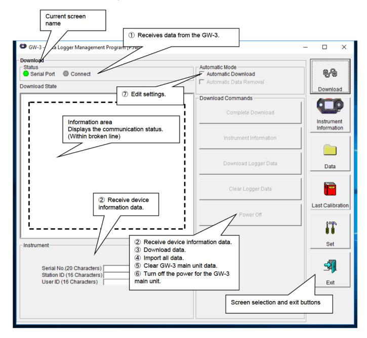
To start data communication, place the GW-3 in a suitable location, start this program, and power on the main unit. The program will automatically determine whether data communication is possible; if so, it will enter reception standby mode.
