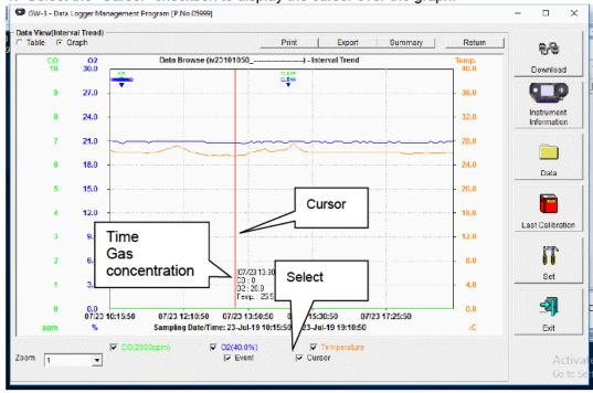
Use the " $\leftarrow$ " and " $\rightarrow$ " keys to move the cursor left and right. Use the " $\uparrow$ " and " $\downarrow$ " keys to move the time and concentration display up and down.
