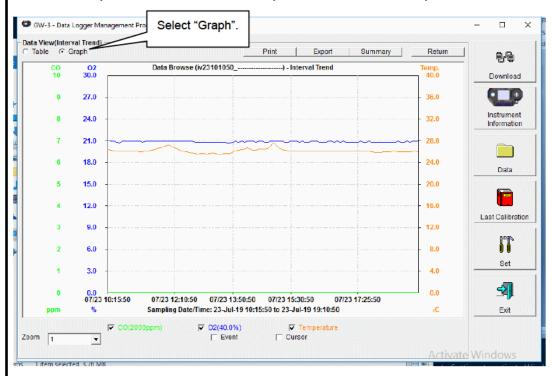
Various operations are available using the checkboxes and combo boxes at the bottom of the screen.
